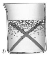
If milk is left to stand for a while in a vessel, the fat will rise and form a layer of cream on the surface because fat globules are not only the largest particles in the milk but also the lightest density. Why use High Pressure Homogenization?
