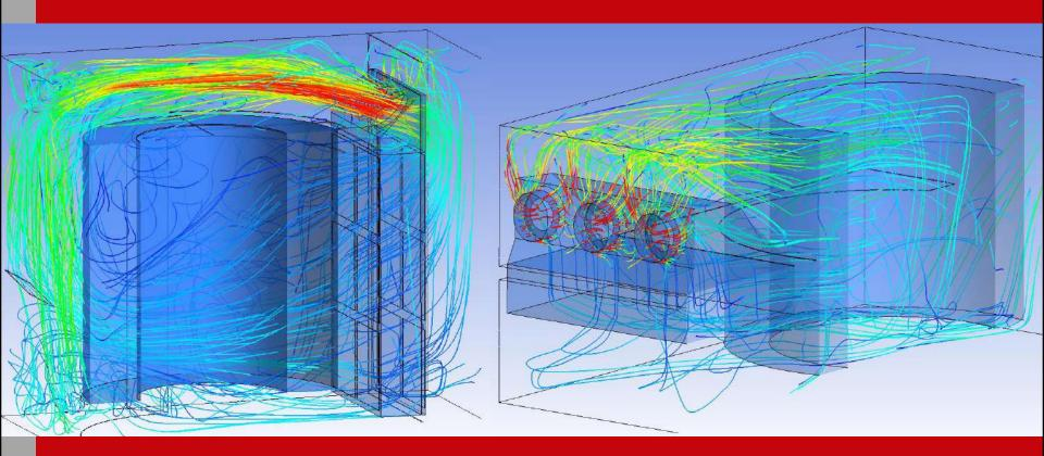
Predicting performance of a freezing system begins with a solid model of the blast freezer
