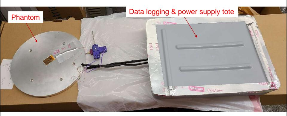
The Phantom is an instrument that simulates the product being frozen for the purpose of gathering heat transfer data within the operating blast freezing system
