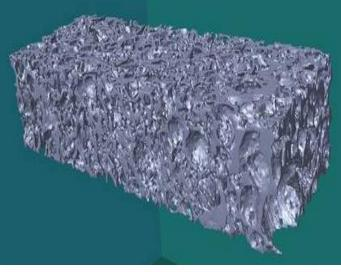
2D shadow images Pixel:  $\rightarrow$  X-ray transmission 3D volumetric data : Voxel  $\rightarrow$  local density
