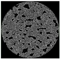
Fast freezing (18.4 °C/min)
